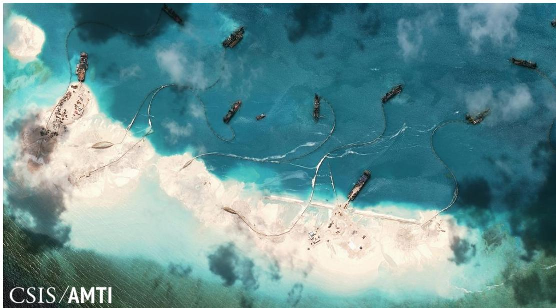
Fig 15: Mischief Reef. This image taken 17 March 2015 shows several dredgers working simultaneously. Picture source is DigitalGlobe, available via the CSIS Asia Maritime Transparency Initiative <http://amti.csis.org/mischief-reef/>.
