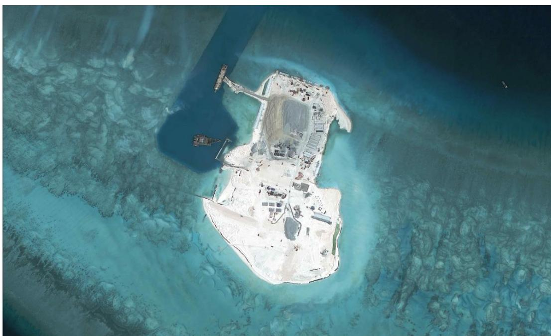
Fig 19: Cuarteron Reef. Image taken 24 September 2014 shows land reclamation in progress and wide dredging track cut into the reef. Picture source is DigitalGlobe, available via the CSIS Asia Maritime Transparency Initiative <http://amti.csis.org/cuarteron-reef-tracker/>.
