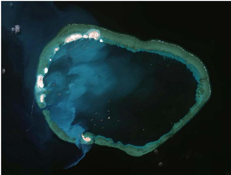
Fig 13: Sediment plumes can be seen engulfing almost the entire western half of the lagoon and the sea beyond the western reef rim of Mischief Reef in this image taken 16 March 2015. Picture source is DigitalGlobe, available via the CSIS Asia Maritime Transparency Initiative <http://amti.csis.org/mischief-reef/>.
